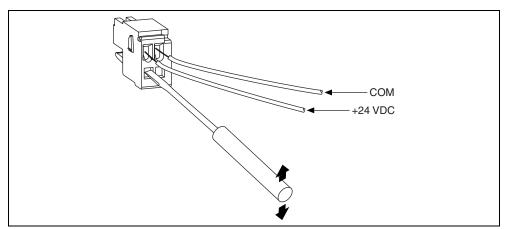
Figure 3. Power Two-Position Header Wiring Diagram
